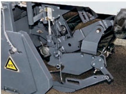
Scanning the surface in front of the milling drum using a wire-rope sensor (optional).
